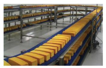
Intermediate Drive (i-Drive) technology is a unique drive system that can engage the belt in the carryway and returnway. With i-Drive technology, you have the freedom to run a single belt for long distances without transfers.
